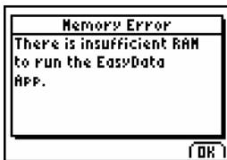
A minimum of 1600 bytes of free RAM is required to start the EasyData application.
