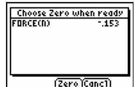
3. When the displayed reading stabilizes, select **Zero**.
