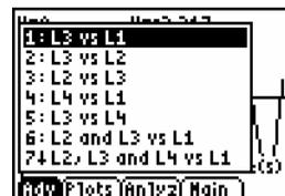
**Plots** When multiple sensors, motion detectors, or photogates are used to collect data, the Plots menu lists all possible data plots that can be graphed.
