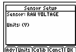
4. Press **CLEAR** to clear the long sensor name. Type in the name of the custom sensor, then select **Next**.
