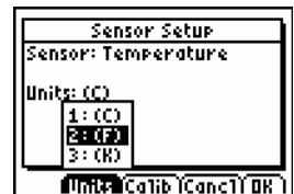
4. The Sensor Setup screen shows the selected unit. Select **(OK)** to return to the main screen.
