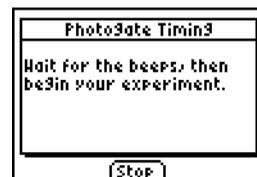
The time required for the pendulum to pass through the photogate three times (a full period) is displayed along with the trial number. Allow the pendulum to continue oscillating to collect multiple periods.
