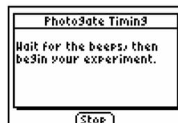
The time required for the cart to pass from the first to the second photogate is displayed along with the trial number. Pick up the cart and place it at the top of the ramp. Pass it through the photogates several more times.
