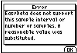
The sample interval or # of samples entered is not supported by the current hardware/software combination. The closest, acceptable value has been substituted.
