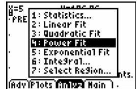
**Power Fit** – This fit is calculated in the form  $y = a*x^b$ . Values for **a** and **b** are calculated and displayed. A minimum of 2 data points is required and all data points must be positive, non-zero values.
