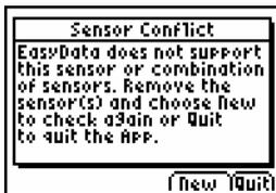
Either the connected data collection device or sensor is not supported by EasyData, or the sensor combination is invalid.
