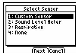
3. Raw Voltage is displayed as the default sensor setup. Select (Adv) to edit the sensor setup.
