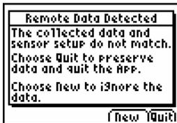
The calculator and connected data-collection device do not share a remote data collection configuration. When remote or long-term data collection is started, EasyData assigns a unique ID to both devices. Only the calculator and data-collection device that share the same ID can be used to retrieve the data.
