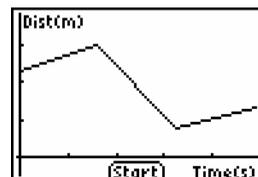
Walk back and forth in front of the motion sensor to match the displayed graph.
