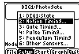
The default **Motion Timing** settings are displayed. The default device should be set as a Vernier Picket Fence. Select **OK** to return to the main screen.
