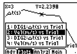
**Options:** When collecting data in Pulse Timing mode, it is possible to use one or two photogates. The example above describes the use of a two photogates. When performed with a single photogate, time is measured between two consecutive blocks of the gate.
