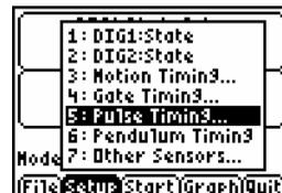
The Gate Distance is displayed. Press **(CLEAR)** and type in the distance between the photogates. Select **(OK)** to return to the main screen.
