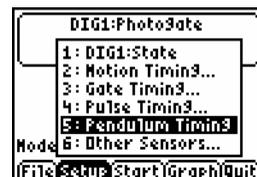
2. Select **(Start)** to begin collecting data. Wait for the data-collection device to beep, then release the pendulum so that the bob passes through the photogate.
