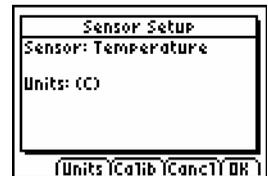
3. A menu is displayed showing the possible units for the connected sensor. Select the unit that you want EasyData to use.
