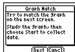
4. A graph of distance vs. time is displayed. The graph should be examined before attempting to match the graph. When ready to perform the match, select **(Start)** to begin collecting data.
