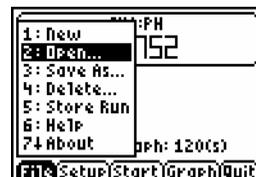
2. The Open Experiment screen is displayed. Select the experiment to be opened and then select **OK**.
