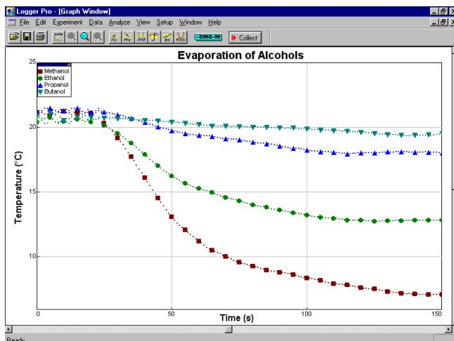
Using four temperature probes to investigate the evaporation of alcohol with Logger Pro.
