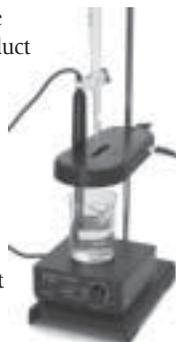
The Drop Counter can also be used for conductimetric or potentiometric titrations using our Conductivity Probe, Ion-Selective Electrodes or any electrode with a 0- to 5-volt output. You could even use it instead of a utility clamp anytime you need to hold an electrode in place.
