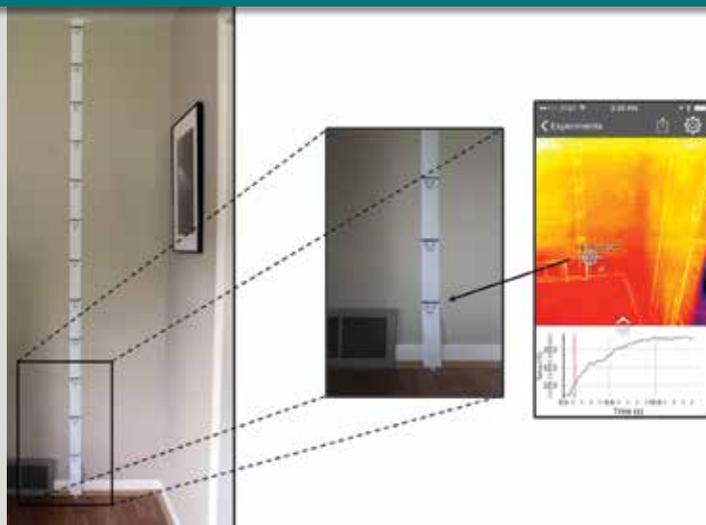
In the “Investigating Thermal Stratification/De-stratification in Buildings” experiment, students use the FLIR ONE™ Thermal Camera for iOS (FLIRONE-IOS, \$249), available from Vernier, and the free Vernier Thermal Analysis app to study thermal stratification and destratification of air in a room.
