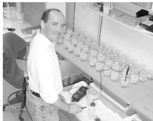
Kevin LaVigne tests soil samples using the Vernier pH Sensor and LabPro.
