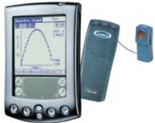
You can use Data Pro in or out of the classroom. In the classroom, a student lab station can consist of a Palm handheld, LabPro, and a sensor. Outside of the classroom, the handy Palm-to-LabPro pouch provides an all-in-one unit for collecting data at your favorite stream or at a local amusement park.
