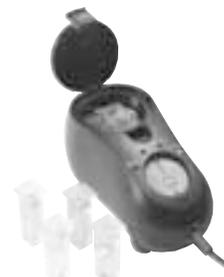
One of our most popular sensors for chemistry, biology, and water quality testing is the Vernier Colorimeter. Our new Colorimeter has the following new features:
