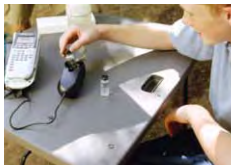
Measuring turbidity of a stream sample
