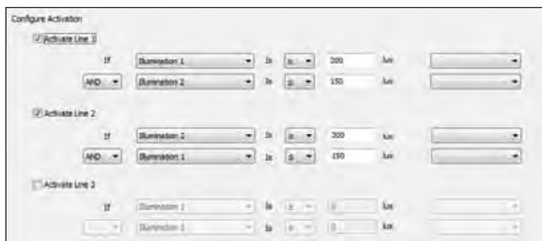
Configuring output logic using the Digital Output feature of Logger Pro
