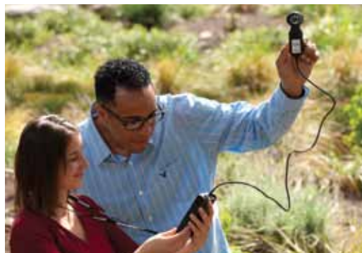
Using the Anemometer to measure wind speed
