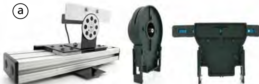
Collecting intensity vs. position data for a diffraction pattern
