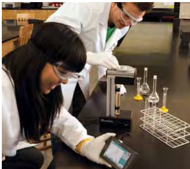
Analyzing the optical rotation of sucrose using the Polarimeter and LabQuest 2
