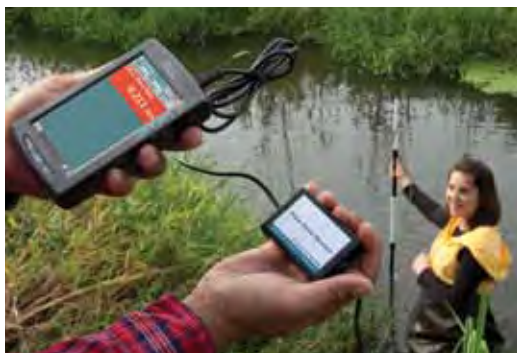
Collecting flow rate data with a LabQuest
