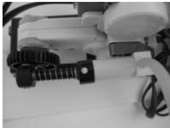
Figure 2. The LEGO Pneumatic Hand Pump connected to an NXT motor
